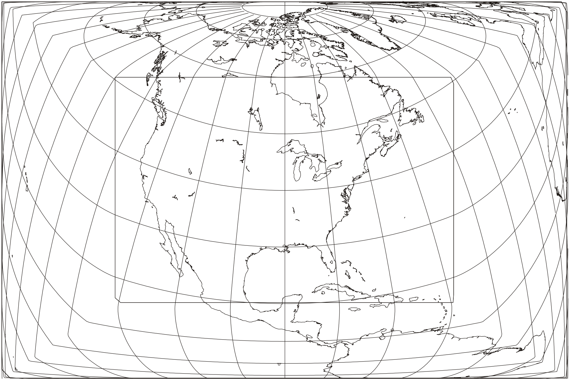
Rectangular "Magnifying-Glass" Tapered Azimuthal Equidistant; Neither Conformal nor Equal-area; John P. Snyder; 1987
