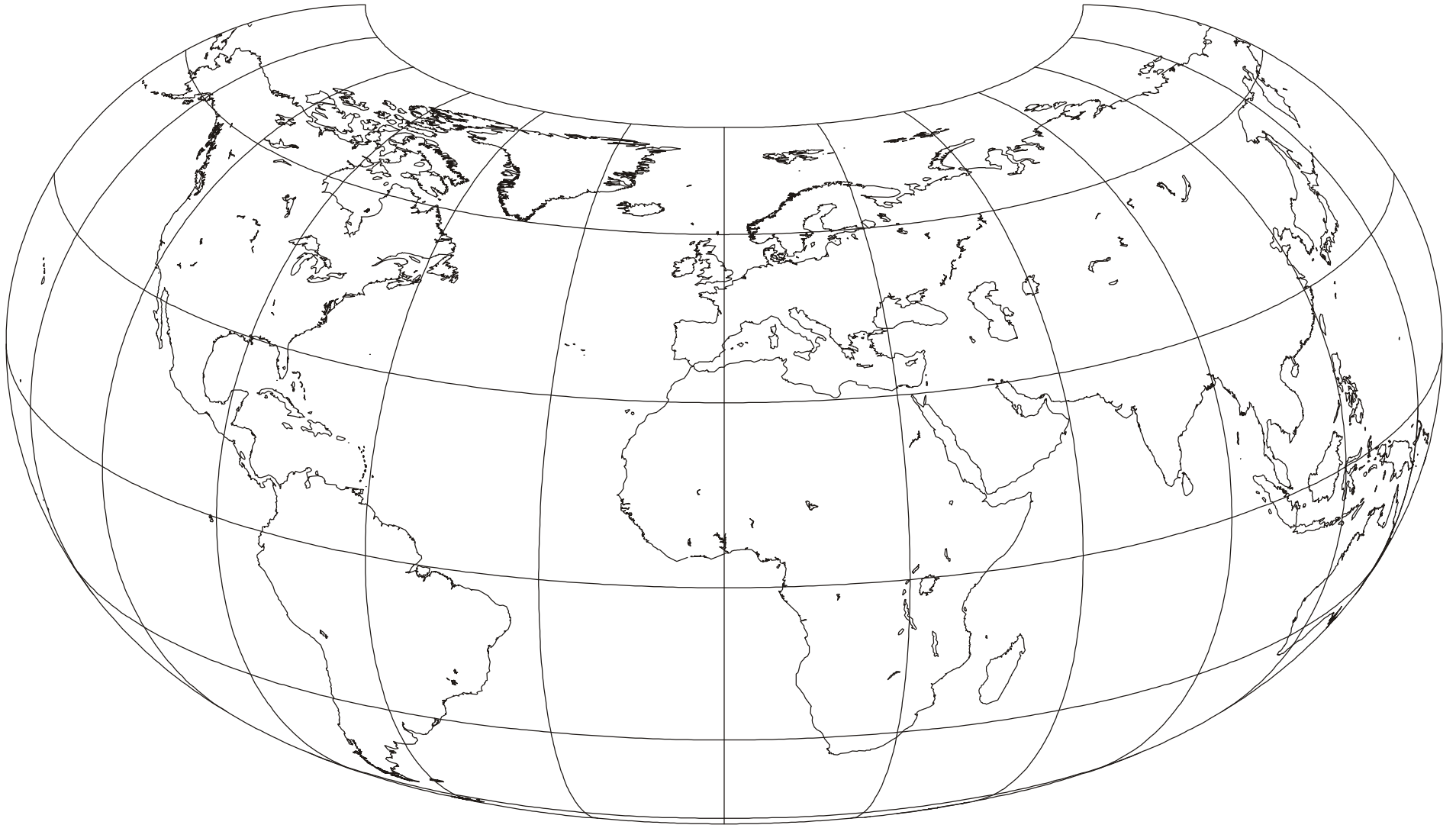
Raisz Armadillo projection; Miscellaneous; Orthoapsidal; Neither Conformal or Equal-area; Erwin J. Raisz; 1943
