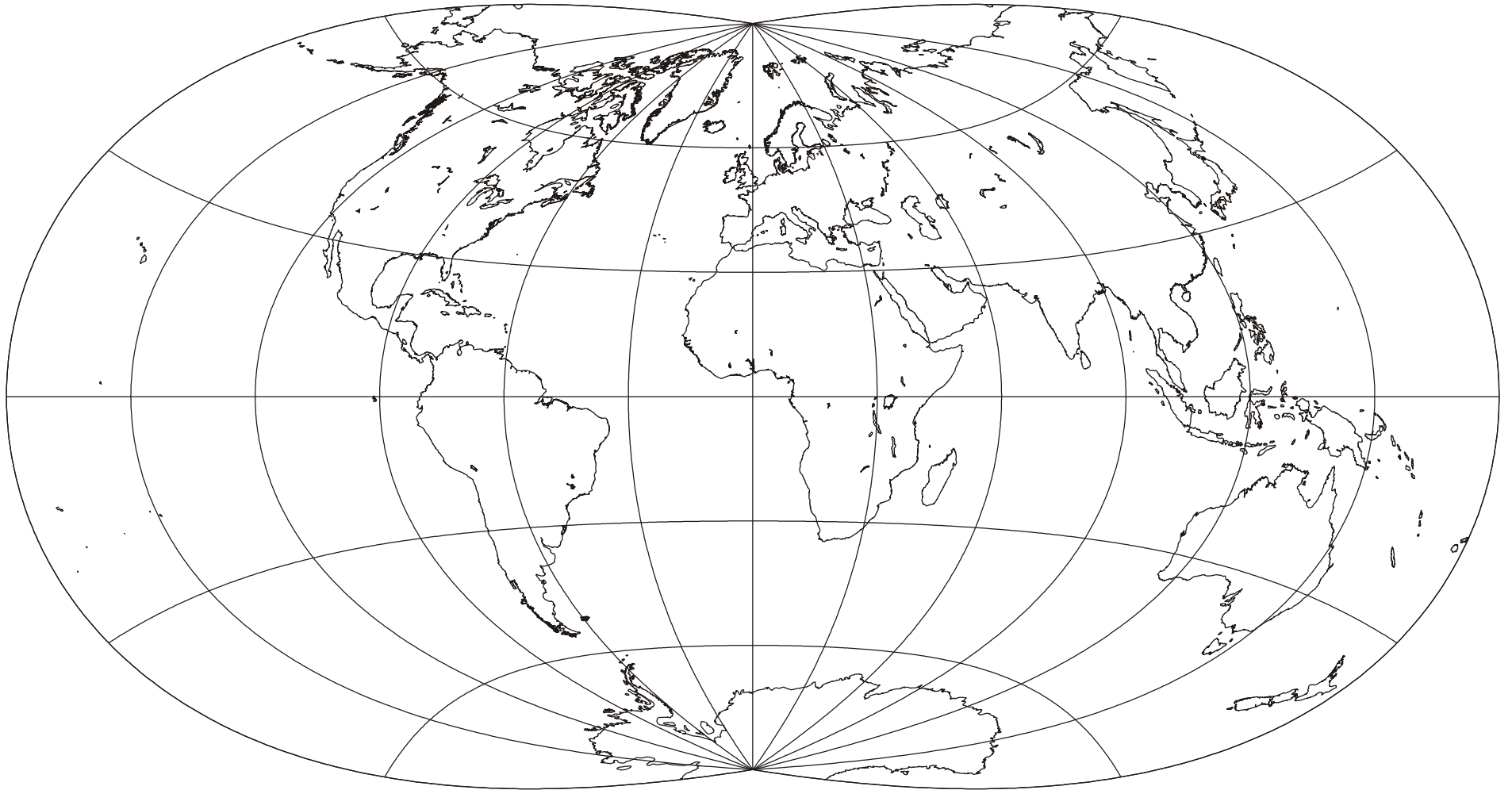
Low-error Polyconic; (with pole as point, twofold symmetry, equally spaced parallels, and correct ratio of axes); Neither Conformal or Equal-area; Frank Canters; 1989, 2002
