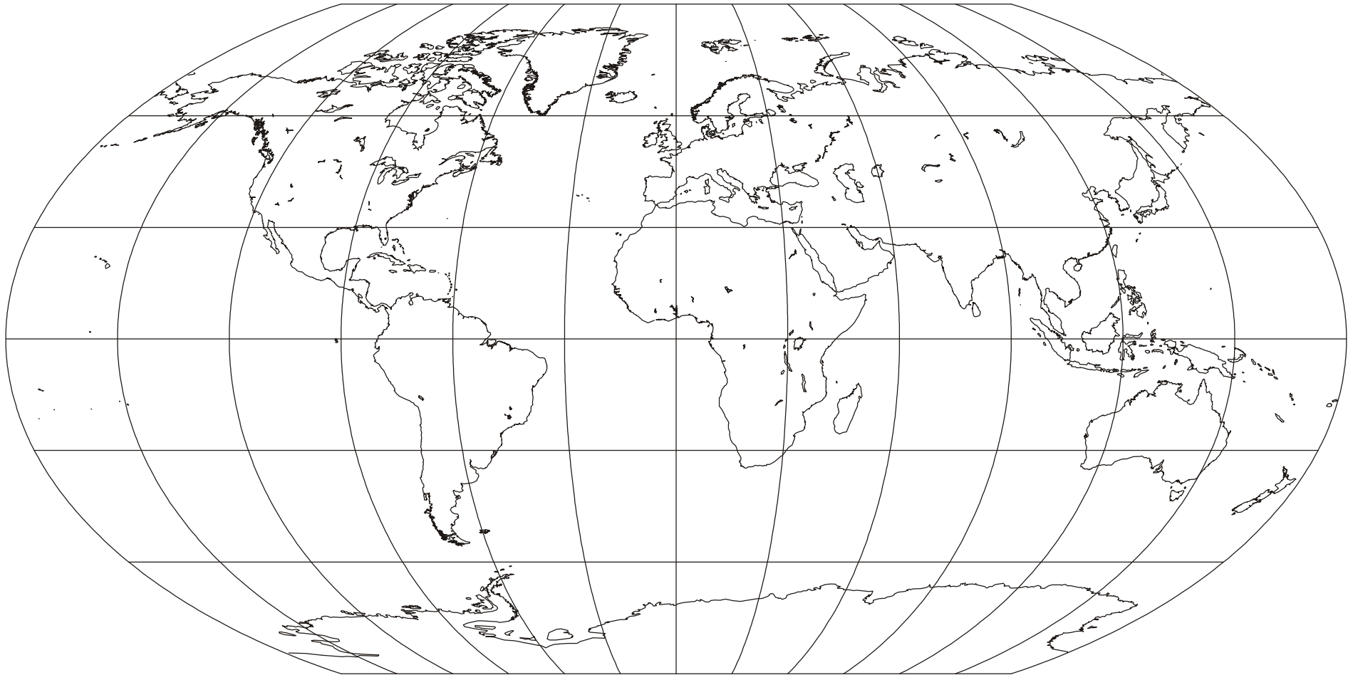
Wagner VI projection; Pseudocylindrical; Neither Conformal nor Equal-area; K. H. Wagner; 1932; R. V. Putnins (P'1); 1934
